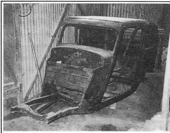
Stripped down ready for sand-blasting.
