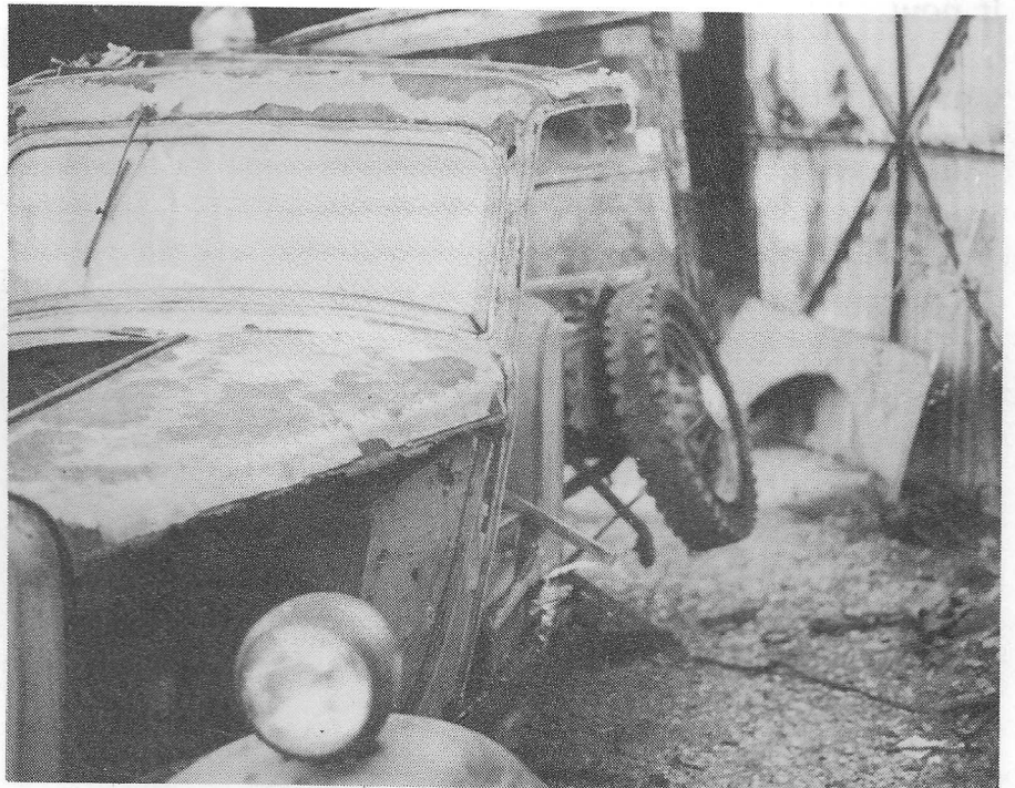
"The nearside had fared worse in the weather. This was the result of jacking up the rear axle!"
