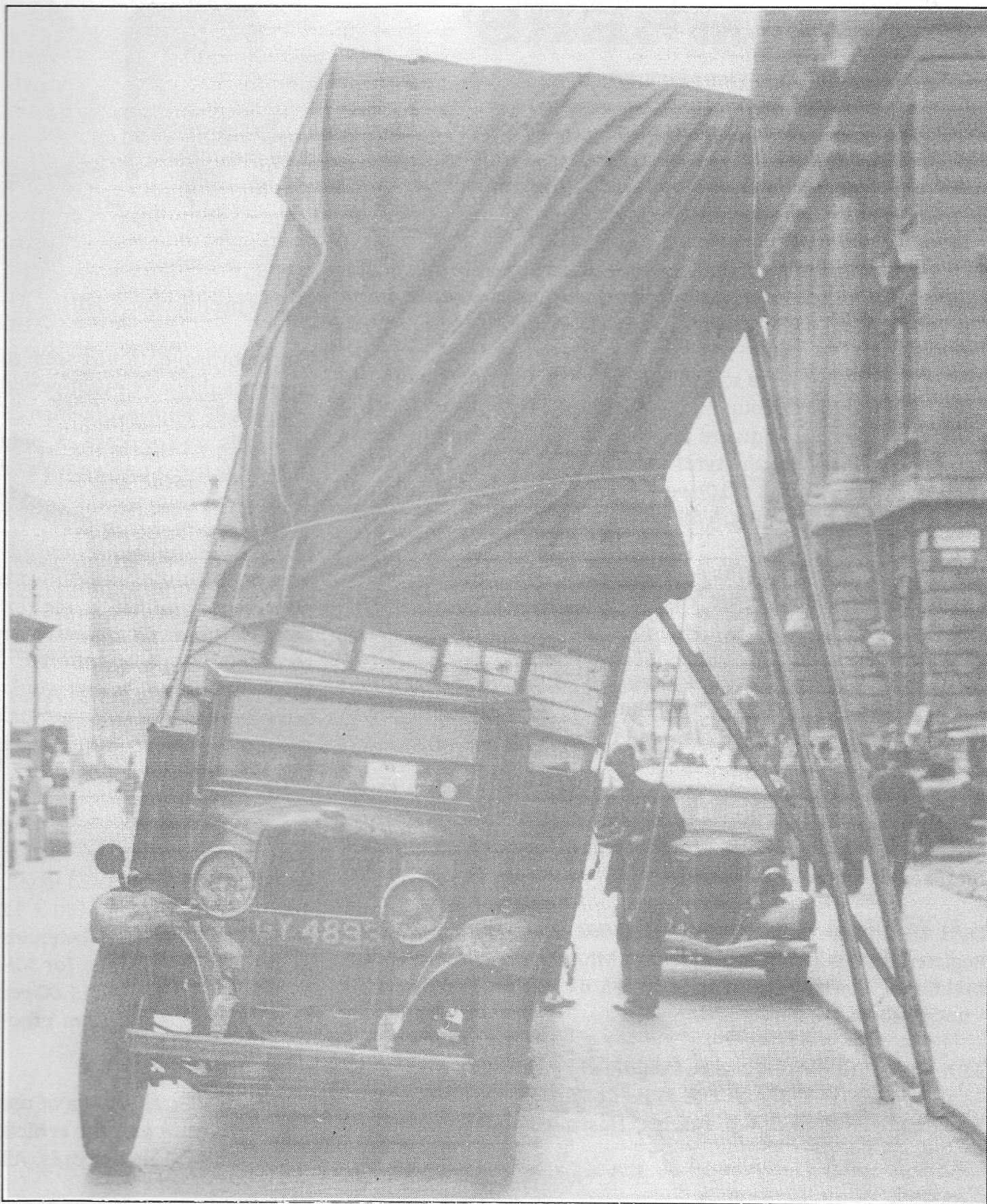
A photograph sent in by Steve Young with, on the reverse "A Moving Story. This cargo shifted in the journey up Regent Street, and props were placed in position to prevent an accident 29.9.39". Note the rather tired looking Model Y parked behind, with a replacement, non-Ford, bumper; awry number plate and "blackout" headlamps; this photograph having been taken during the first few weeks on the Second World War.
