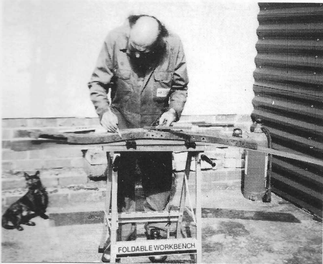
"Marking out the new chassis sides on plywood."
