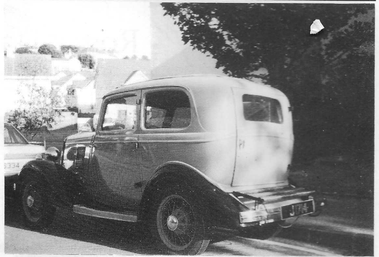
"The rear view of John Follon's Model 'Y' showing the Jennings rear door conversion."
