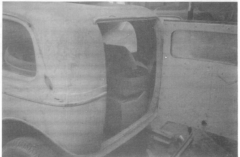
The rear door open. Note the rain ridge above the door
