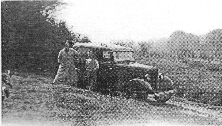
"Mother and son, in school uniform, standing by short rod Tudor Model 'Y', probably in the mid '30s. AKM 298, registered in Kent in June 1933. Note the makeshift luggage rack bolted under the vinyl roof, which would not have enhanced the waterproofing!"
