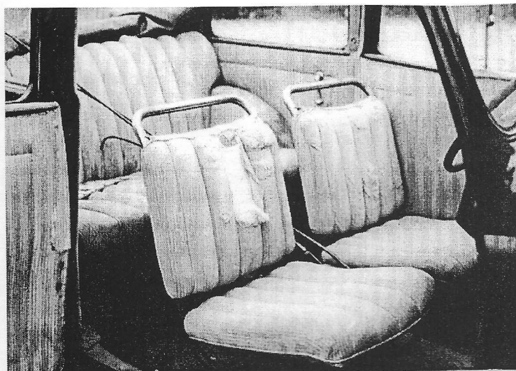
"A typical seat design with handrails on Köln manufactured cars. The passenger seat rocks forward to gain access to the rear. It is presumed that the driver's seat has adjustable leg room. Photographs courtesy Jim Oliver."
