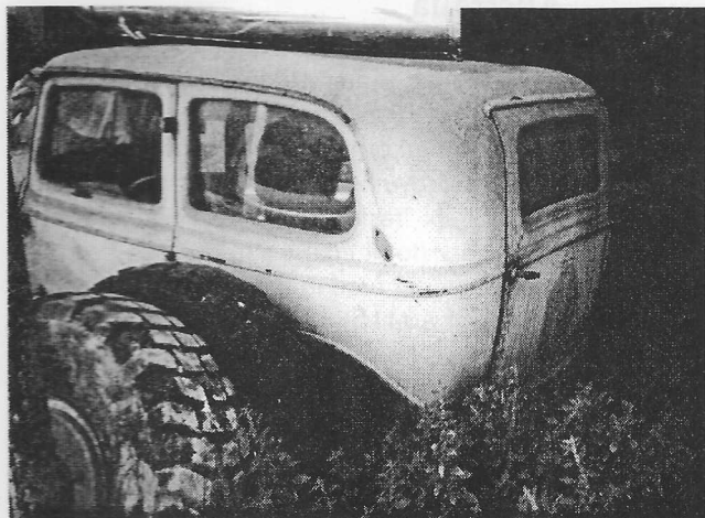
"The Jennings door at the rear of the Tudor Model 'Y'."
