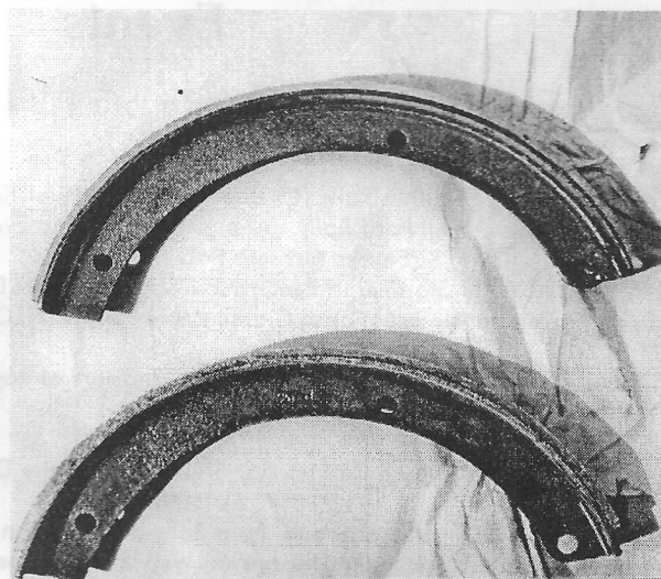
"The early (1932/33) and 'not so early' (1934) brake shoes showing the addition of the reinforced web at the rollers' end."
