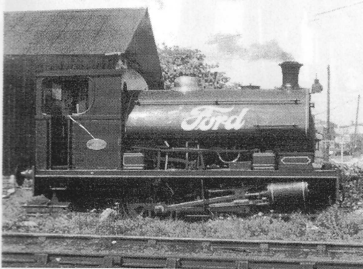
The Peckett & Co. R4 class 0-4-0ST, No.6, simmers outside its shed at Briggs Bodies Ltd., where it was out-stationed. Briggs' sidings lay on the far side of the Tilbury main line, so servicing required a trip across the tracks to the home shed. No.6 was scrapped in 1965.
