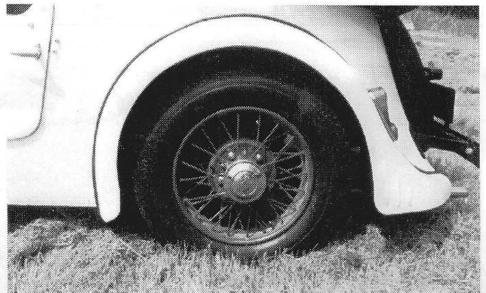
One of the 5.50x16 inch, 50 adjustable spoked wheels on David and Wendy Grace's Model 'Y' Arrow Alpine.
