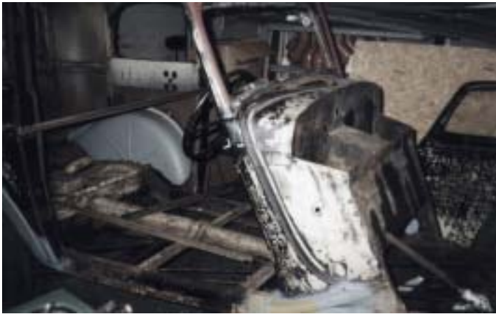
The body shell of Ian MacDonald's September 1934 cream Model 'Y' revealing the cream underpaint on the floorpan and externally, as the black is rubbed off."
