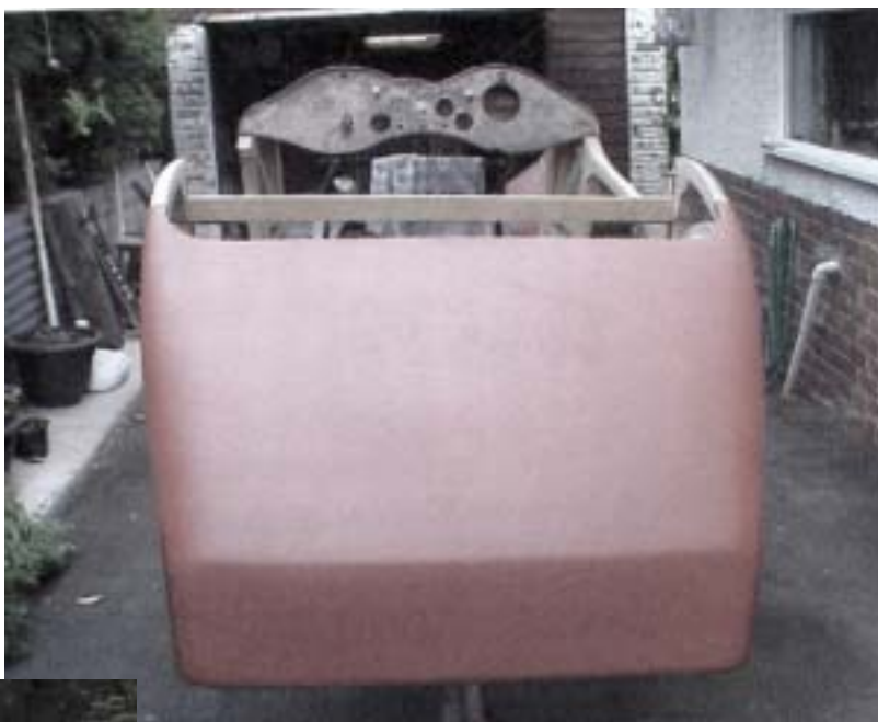
The re-skinned rear end. It has been decided to do away with the opening boot as it leaked badly and contained very little space once the spare wheel was inside.
