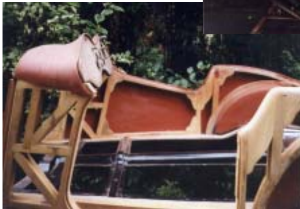
The inside of the new panel showing the superb craftsmanship of the woodwork.
