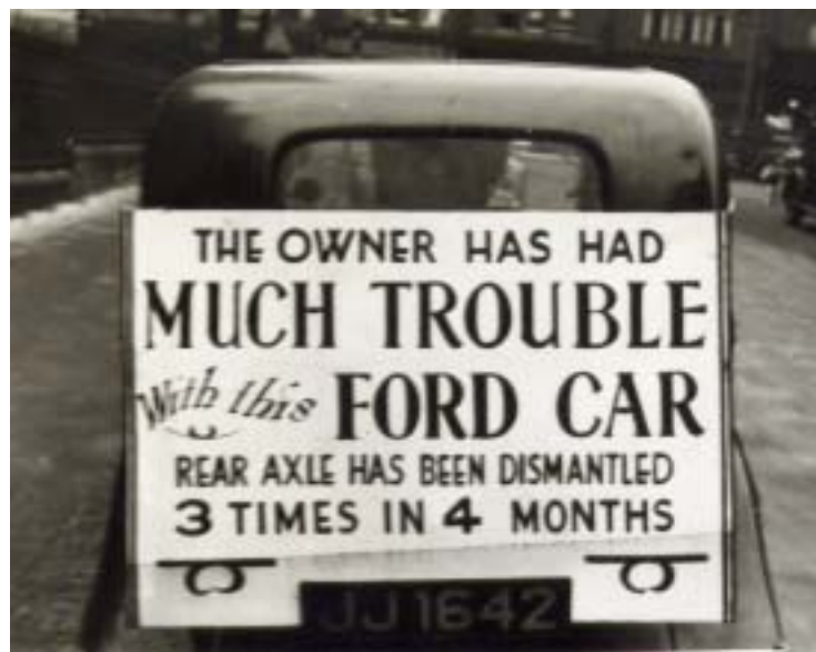
Early short rad Model 'Y' parked in London street. The owner waging his one-man war against the Ford Motor Company for its failure to solve his rear axle problem. This was the only major design fault in the hastily developed Model 'Y'.
