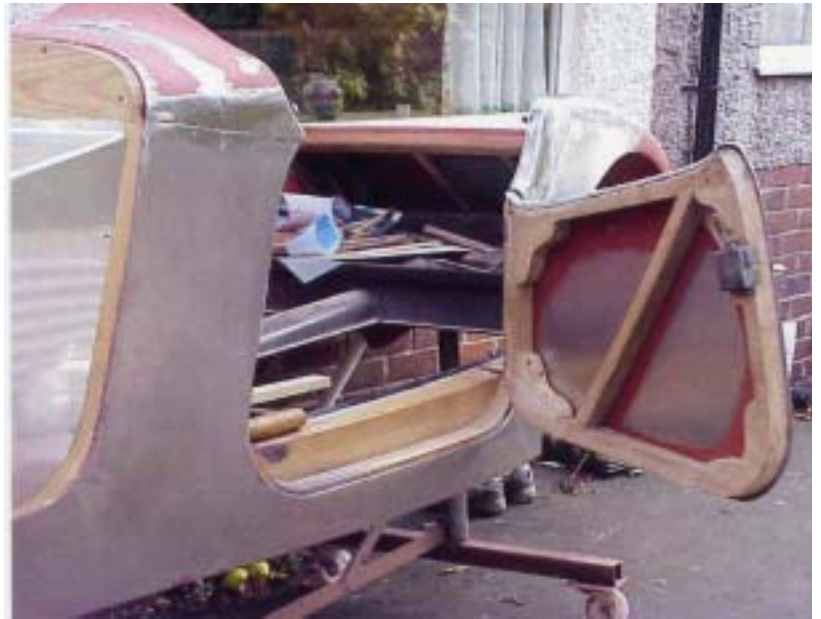
The expertly crafted near-side door, showing the outer skin folded round the inner skin.
