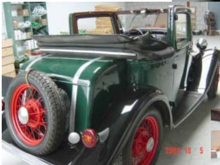
The rear of the coupé showing the rounded back of the body tub and the add-on looking boot. This is identical to the design of the ex-Graham Tomlinson's Kelsch.
