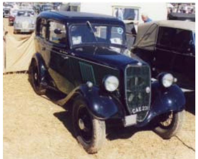
Mike Workman's trials Model 'Y', with fan assisted cooling and extraction tow ring at front in lieu of bumper. Other modifications are hidden in this photograph!
