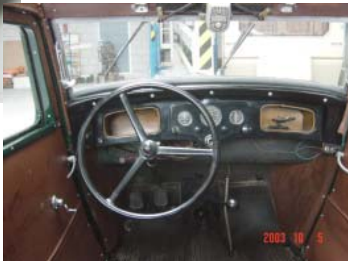
The left hand drive interior of the Kelsch coupé. Note the larger than standard distance between the glove compartments and the sides of the car, due to the wider body shell to the rear of the bonnet sides.
