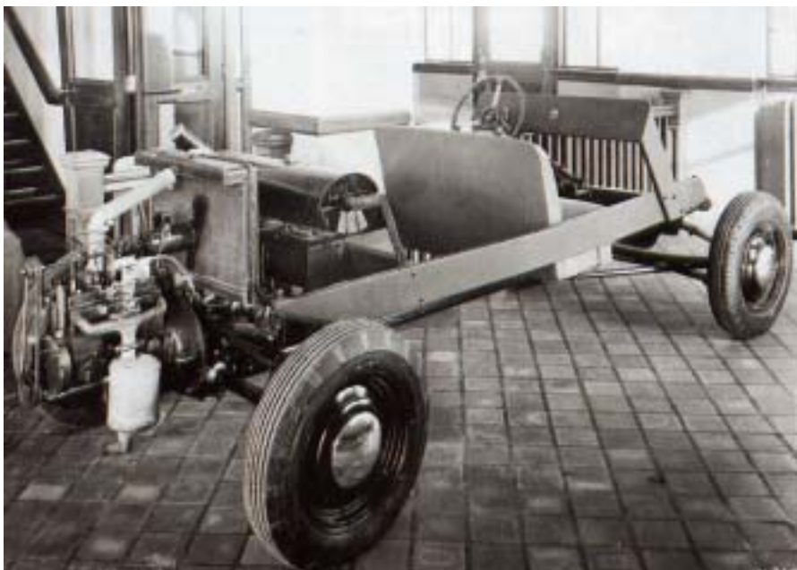
A mock-up of an experimental rear engined Ford designed in 1940 in Dearborn. Note the 'Baby Ford' engine; probably left over from the Model 'C' development programme.
