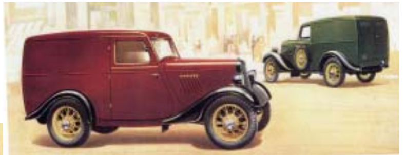
Extract from 1937 'Ford Commercial Vehicles' brochure showing spare wheel on nearside door.
