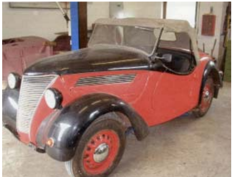
The recent find in Germany. Note the dipped doors and Model 'C' type headlamps indicating an earlier design of Eifel roadster.
