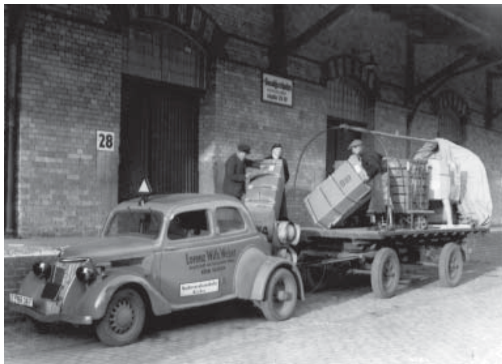
A fascinating photograph of a modified Eifel saloon being used as a tractor during the war in Germany.
