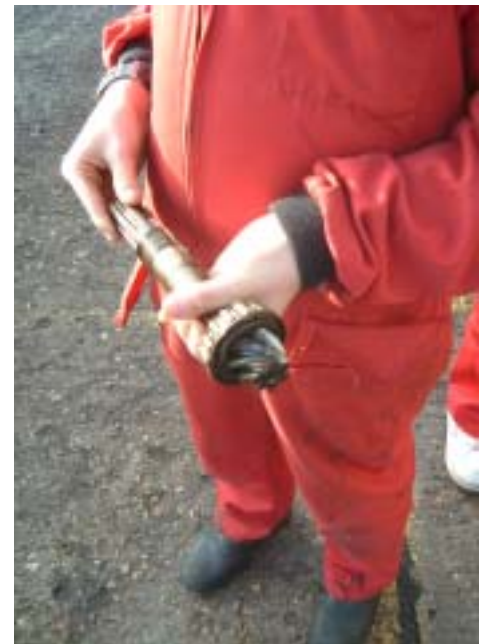
The chewed pinion with one and a half teeth missing. Obviously not the One Armed Bandit holding it, but Alistair.
