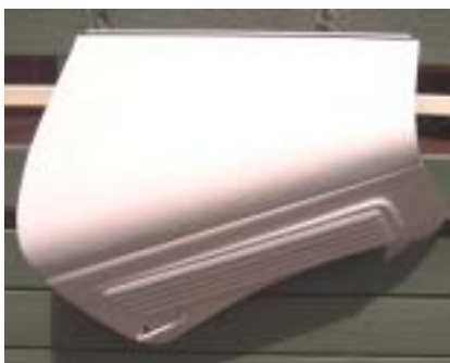
Cyril Johnson's primed bonnet showing clearly the taper of the swage line from left (scuttle end) to right (radiator grille end) and the taper in the protrusion of the vent from right to left.
