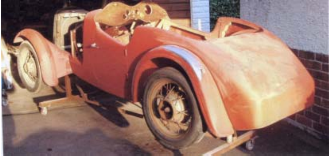
The rear wings expertly manufactured and fitted by Terry.
