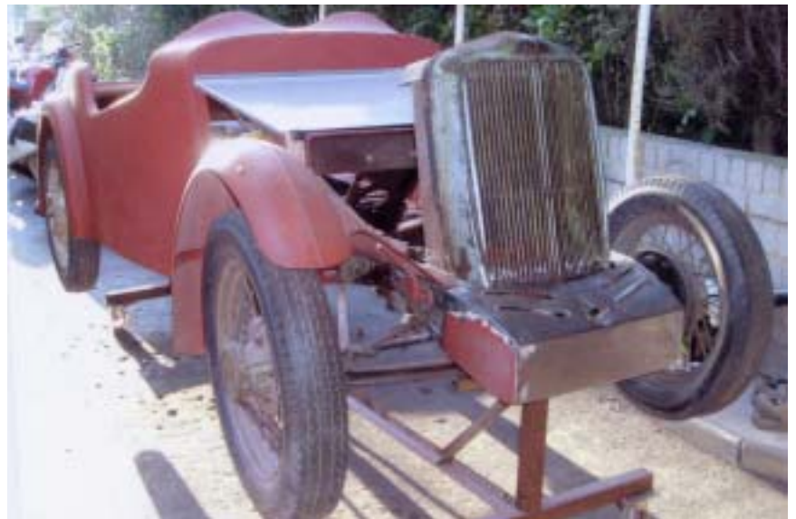
The repaired radiator grille in situ with the unique front valance of the Bezzant.
