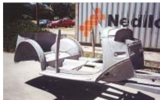
The cut down donor car after sandblasting.
