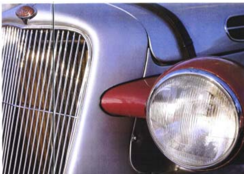
The Model 'CX' bonnet with red Edfor grille badge. Note that the chevrons on the grille are thinner than on the English 'CX' and German Eifel.
