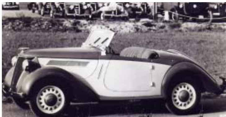
The Ford Köln 'original' photograph of the 1938-1940 Karmann bodied Eifel Roadster. The collection of Ford chassis in the background include Model 40 trucks and 1938/39 V8 chassis with horizontal chrome strips on the grille, which were peculiar to Germany.
