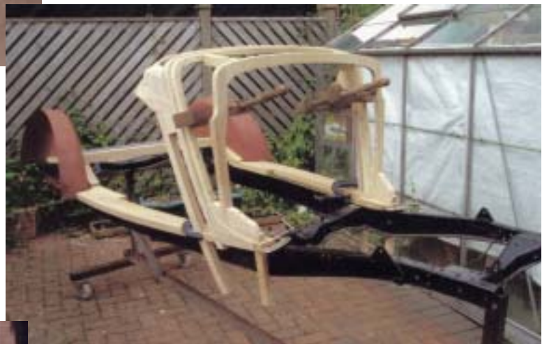
The ash frame taking shape on the repaired and glossed chassis.
