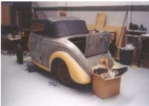
Hood fitted at trimmers.
