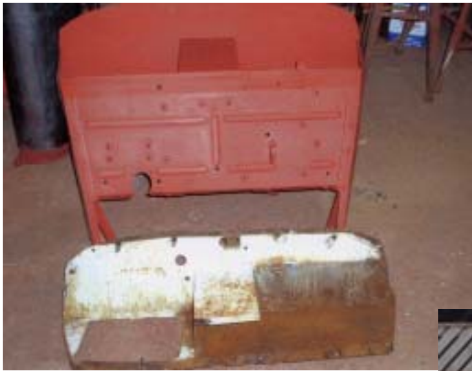
The refurbished bulkhead, with the old, corroded top half sitting on the ground in front."
