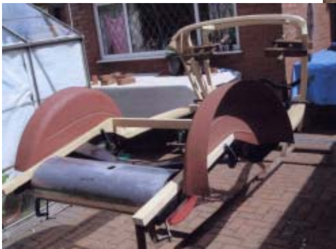
The view from the rear shows the new petrol tank in situ.
