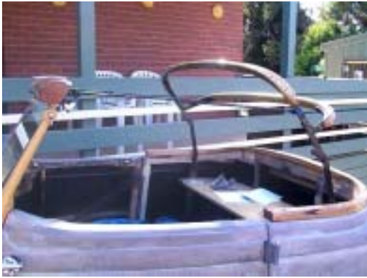
Hood irons and frame manufactured and fitted. Note parcel shelf in rear of tub
