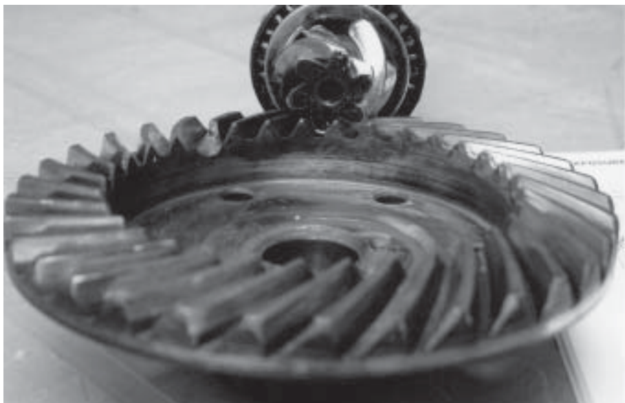
John Keenan's damaged crown wheel and pinion, with half a tooth missing on the crown wheel and the top tooth on the pinion looking decidedly less than complete. Why do they do it to us?
