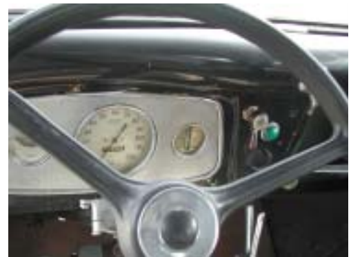
The beautiful Jaeger speedometer and hydrostatic fuel gauge on the inserted instrument panel. Ford France obviously preferred Jaeger to the Dagenham Cooper Stewart speedometers.
