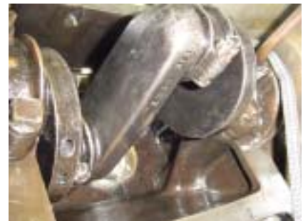
Engine overhaul. Crankshaft with AMBROSIA cast into web.
