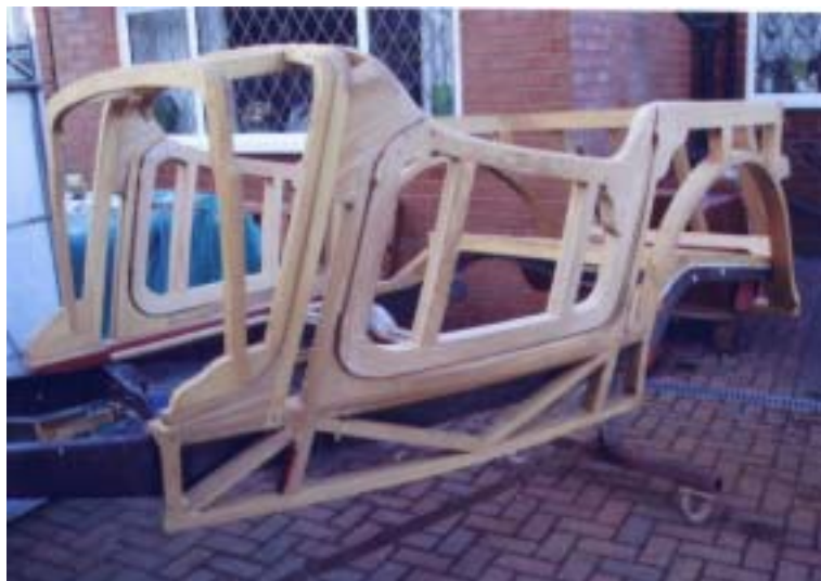
Front quarter view of Alpine frame, with doors fitted. The workmanship is unbelievable.
