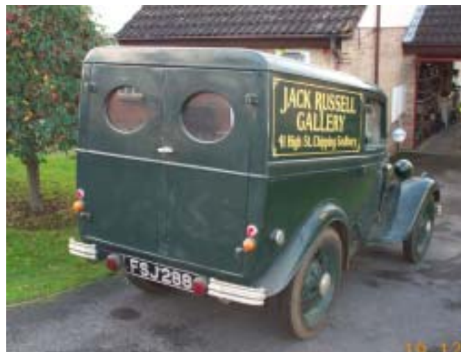
What appears to be a van body on the Tudor short rad saloon chassis, except that the raised swage lines did not cross the rear doors in production. Note also the saloon bumper bars supporting the spurious bumper ends. Production vans did not have rear door windows, but many had them added as a reversing aid.
