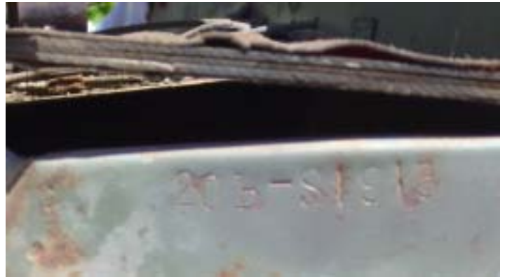
The body number of Andy Leach's 'CX' sedan (20B S1913), which was hand-stamped at the top of the side of the tool box after manufacture of the body at Geelong, Victoria.
