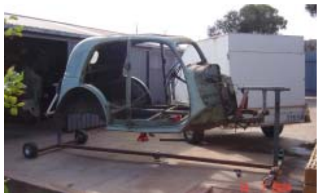
Andy Leach with the bodyshell of his 'CX' sedan on his home-made 'rotisserie' in South Australia
