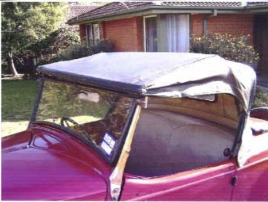
The deep windscreen with black enamel frame on Matthew Watson's "Standard" Roadster (19 R28). Note also the straight-topped doors."
