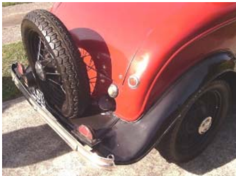
The rear view of Matthew Watson's "Standard" Roadster (19 R28), showing the larger body tub, which bears some resemblance to that fitted to the Australian-built Model A Roadster. Note the petrol filler protruding from the join of the body tub and the rear valance
