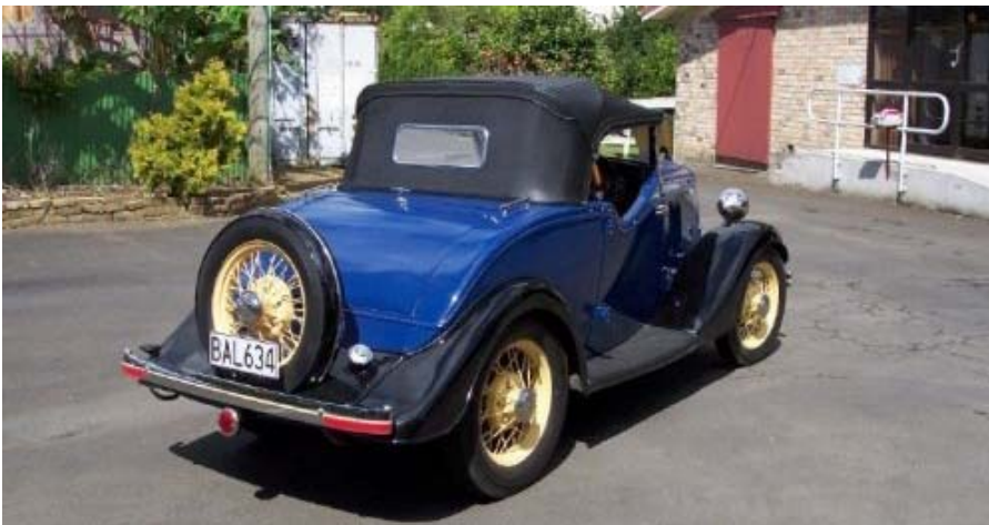
The rear view of Gavin Welch's De Luxe Sports Roadster (now in Auckland, New Zealand), clearly showing the less bulbous, sleek and shortened rear end to the body tub, allowing the petrol filler to protrude through the centre of the rear valance. Note the Dicky seat handle at the top of the 'boot' and the chromed grab handles behind the hood.
