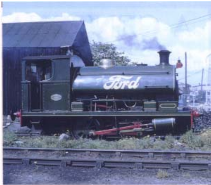
No. 6, the Peckett 0-4-0 ST on outstation duty at Briggs Motor Bodies' sidings in 1961. This replaced old No. 2, a 1901 Hunslet saddle tank (ST), in 1937. These were the only two 0-4-0 steam engines employed by Ford. Note the old logo.
