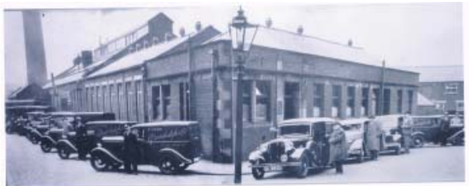
Off a pub wall in Lancashire. The vehicle fleet of Greenhalgh Ltd., Dyers and Cleaners of Burnley, which included eight Model 'Y' vans, the nearest one of which is a post-October 1936 model with its spare wheel on the near-side door.
