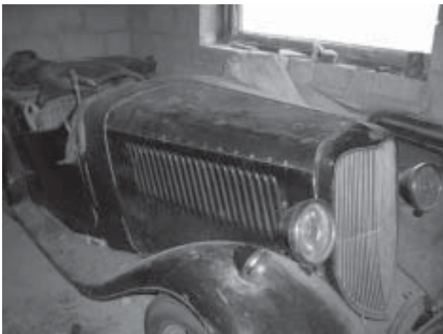
The tell-tale bonnet of the Abbey Coachworks Ltd. body. The 22 equal vertical louvres and the 15 pot rivets along each of the bonnet hinges.
