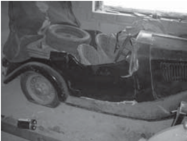
The body tub of the Abbey showing the hood recess behind the door and the non-original, but very period, wicker seats.
