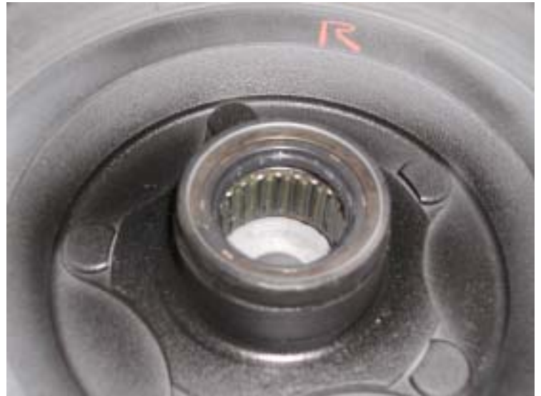
The Club outer sleeved rear bearing fitted into hub.
