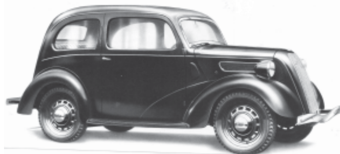
The 8 hp 7Y Ford which was designed by Roberts of Briggs Bodies Ltd. and Patrick Hennessy and which entered production in September 1937.
