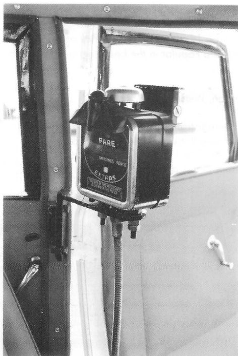
4. The fare meter inconveniently placed in the front passenger door entrance. Note the speedometer cable descending to a take-off point, presumably on the propshaft, and the bell on top of the meter.
