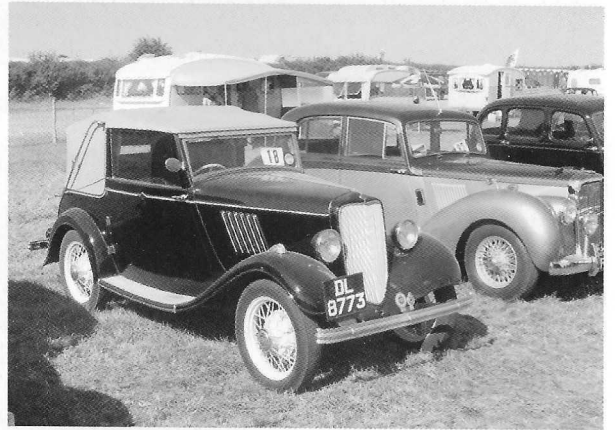
Always a beauty to behold; Robert Stay's Salmons & Sons Ltd.-bodied Cairn coupé with its Tickford hood. The car dates from the change-over period from short rad to long rad. Hence the short rad grille, bumpers and wings and the long rad bonnet.
