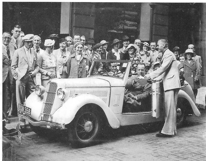
The beautiful looking Jensen bodied drop-head coupé on the Model 'CX' chassis. Note the front hinged, straight topped doors and the Tickford pram-style hood irons. Can anybody tell me the names of anyone present. I suspect one might be a Jensen brother.
