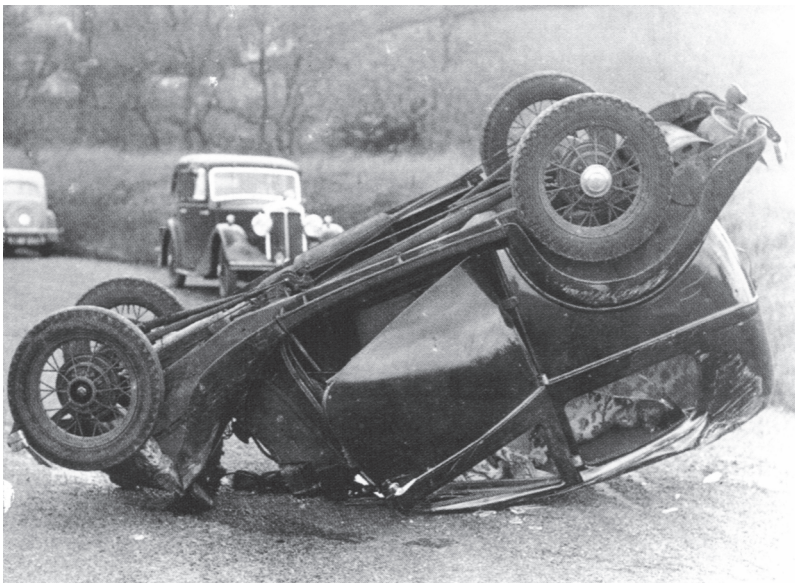
Although the Model 'Y' leans pretty dramatically when cornering at speed, it is quite difficult to roll it. This one appears to have taken a corner rather too wide and taken out a concrete post with its front axle and offside wing, resulting in curtains for what appears to be a rather smart 'Y'."
