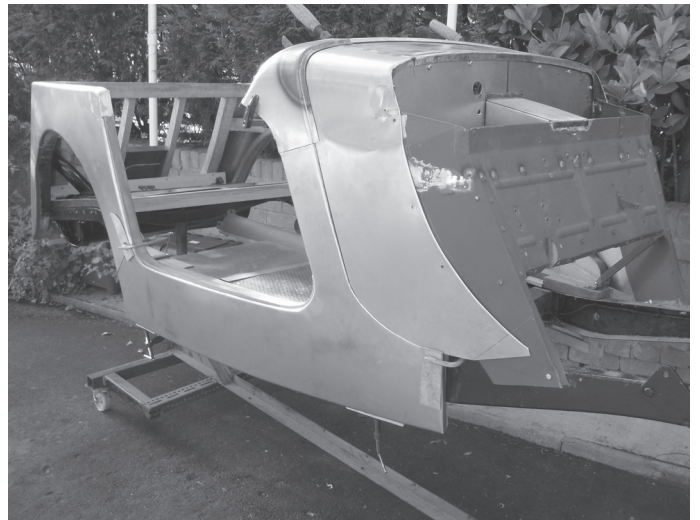
The off-side panels being fitted. Note the completed work on the modified bulkhead and the scuttle.
