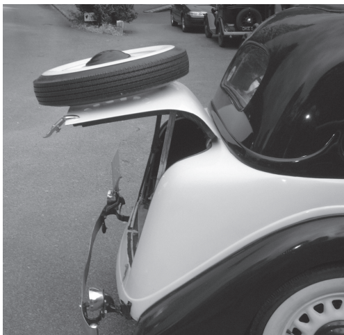
The top-hinged boot on Jim Miles' 1936/37 Eifel. Note the similarity of the latch to that on the Migö boot.
