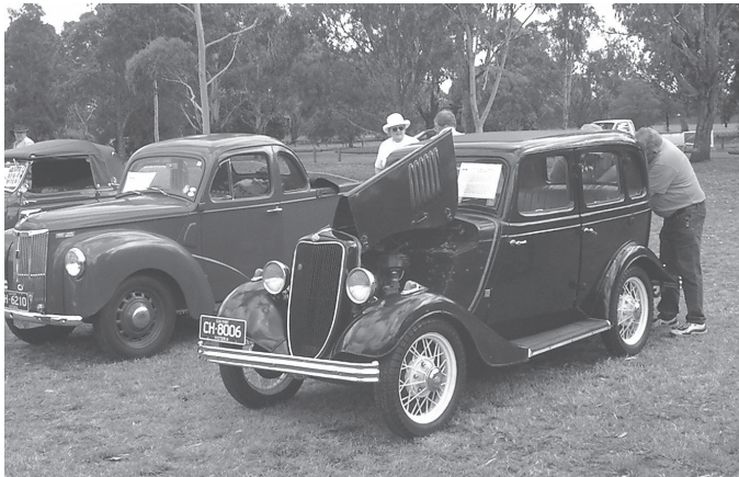
Bernie Bridle with his January 1934 Geelong bodied Fordor Model 'Y'. Note that this early long rad has short rad bumpers. These were supplied with all export long rads (less those to Eire) until the stock was exhausted at Dagenham (approx. March 1934
