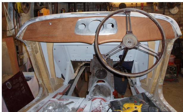
The new mahogany dashboard with the newly crafted mottled aluminium instrument panel fitted.
