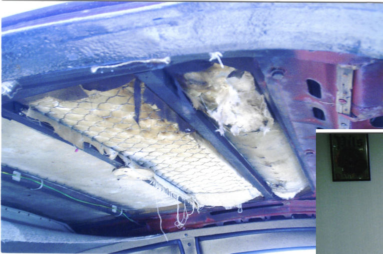
The roof with the burnt headlining removed, showing the singed roof sticks and padding.
