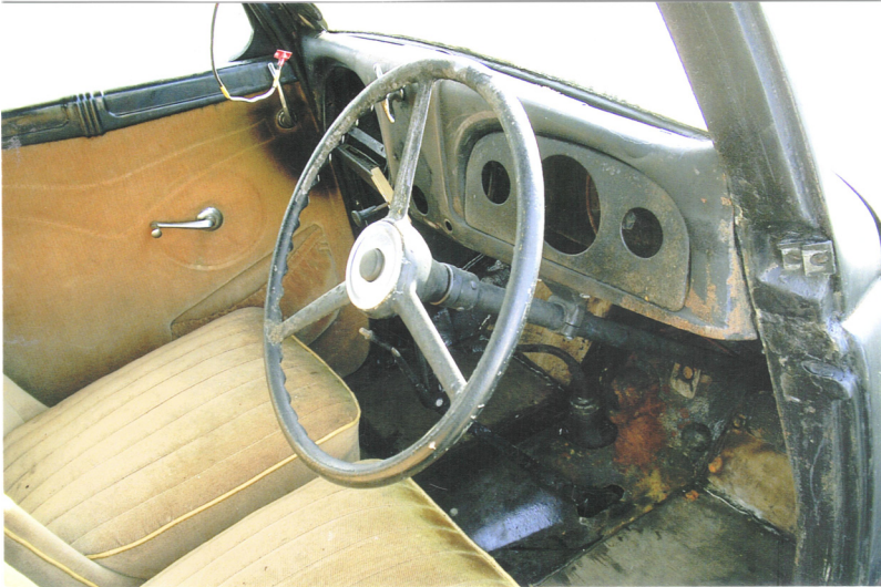
The car as sold on eBay, with fire damage to the door pillar, rear of the dashboard and singed seats and steering wheel. The instruments, rear view mirror and gear knob had been taken.
