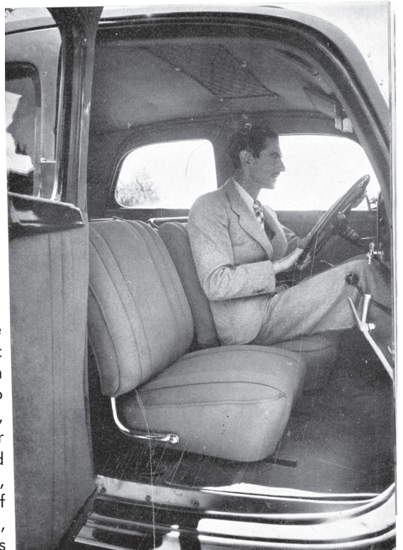
The front of the Fordor 1936 Modelo 10. Note the Cologne-type hinged seats, with a slide adjustment for the passenger, the magazine net above the driver and the fact that the handbrake lever is on the nearside of the gear lever (as with RHD cars). The cloth upholstery would have been locally manufactured in Spain."
