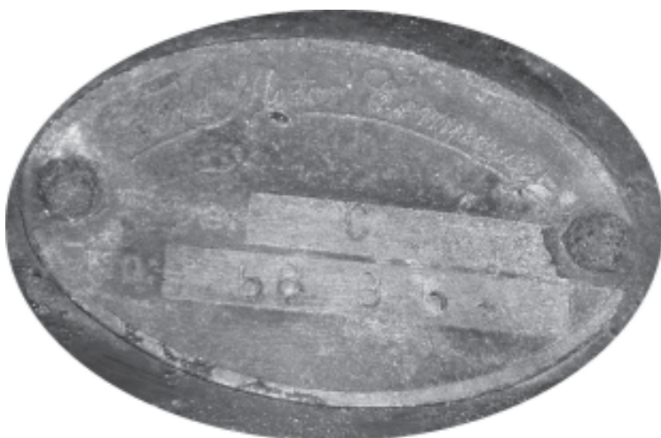
The Ford Copenhagen copper oval plaque, which is riveted to the bulkhead above the toolbox and which reads only 'Ford Motor Company', with blanks labelled 'Type' and 'No.' and on which, in this case, is hand-stamped C and 68864 respectively.
