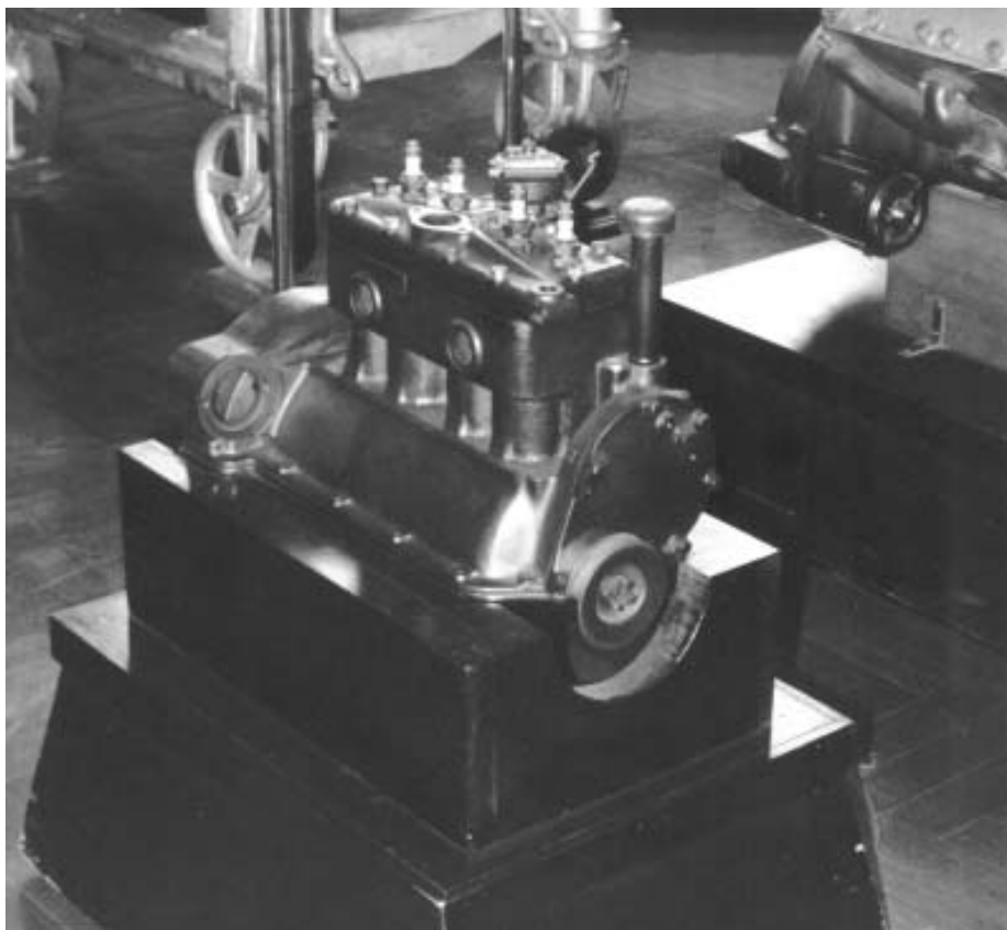
An early experimental Model 19 engine spotted and photographed in the Henry Ford Museum in Dearborn by Luis Cascante in the 1970s. Note the dual water inlets and water jacket at the top of the cylinders only. Enquiries in the late '90s led me to believe that the engine was scrapped in the interim.
