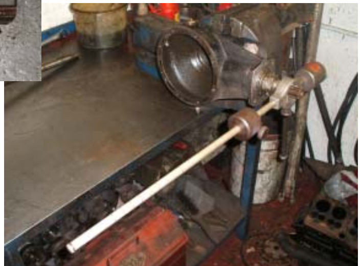
The pinion assembly ready to drop into the heated differential casing."
