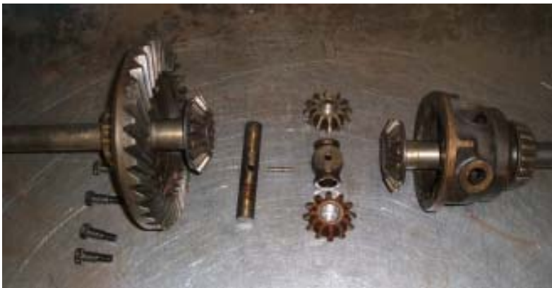
The rear axle split down to its component parts.
