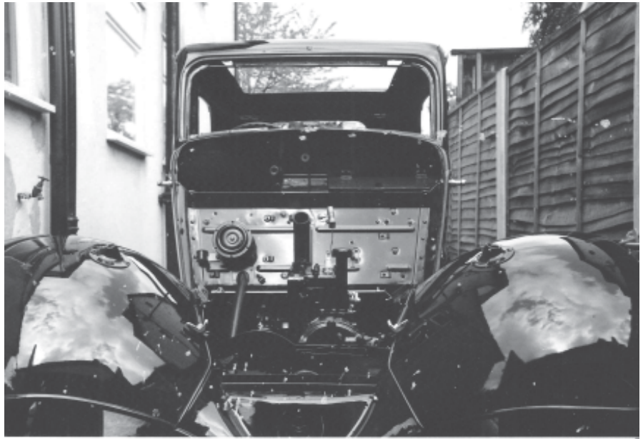
Everything sand-blasted and coming back together again in 1986. The intensity of the 'Taxi' black paint is obvious.
