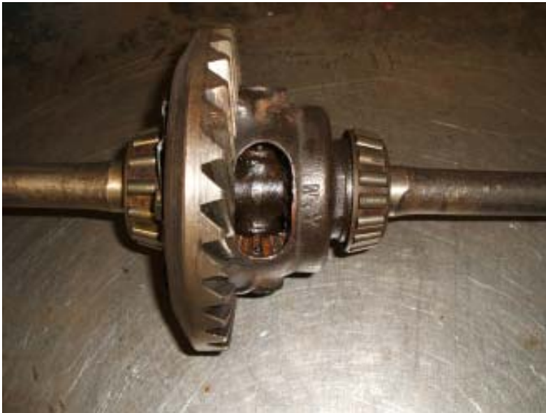
The complete differential and half-shafts."
