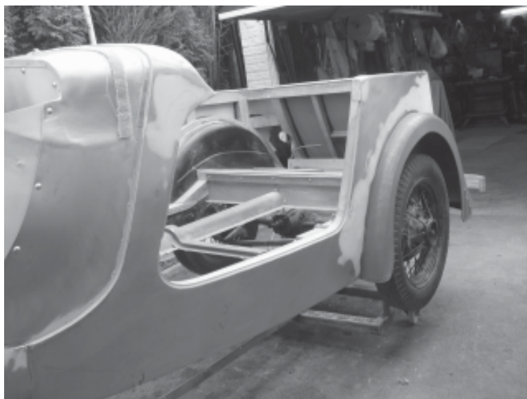
The rear wings symmetrically positioned around the wheels.
