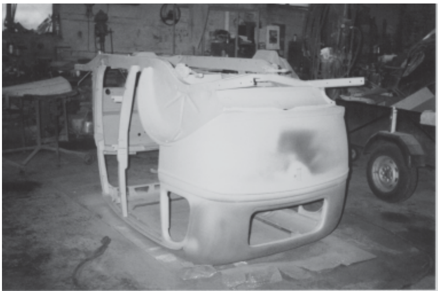
The lower half of the body after acid-etching. Note the superficial rust forming on the upper half (at the bottom!).
