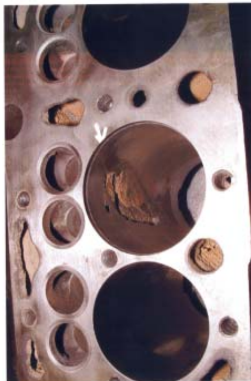
The Model 'C' (Eifel) block out of Jim Miles' roadster after one of the bores had been lightly skimmed. The rust moth had left the walls paper thin. Photograph courtesy Tim Brandon.
