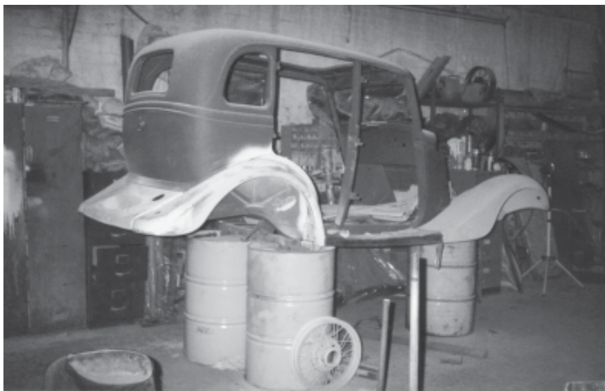
The body, in red primer, with wings and running boards finally and correctly fitted.
