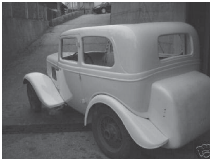
The unrestored Köln as it appeared on ebay. Note the holes in the side of the boot to carry the rear lamps and number-plate bracket. Another of the ebay photographs showed the holes for the spare wheel carrier low down on the rear of the boot.
