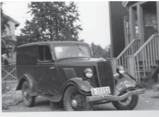
Terje Saethre's father's 1935 van, in which he says "vokste opp i" (I grew up). Note that front bumper bars and a bumper have been added. Also, despite it being a LHD van, the spare wheel carrier brackets are in situ on the nearside door – not the driver's door. Perhaps Briggs Bodies Ltd. couldn't stretch to producing two differing sets of van doors as the demand for LHD vans was minimal.
