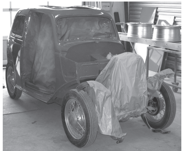
The early style Ford Eifel being restored by Benteler A.G. in Paderborn, Germany, ready to go to the paint shop ('varnisher').
