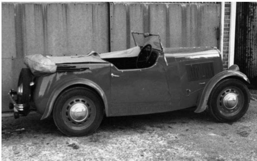
"One of the first Kerry tourers to be bodied by Whittingham & Mitchel, Y1627, built on an October 1933 short rad Model 'Y' rolling chassis. Note the later modification to 'upright Pop' wheels and brakes. The car is now lost to us in Rome.
