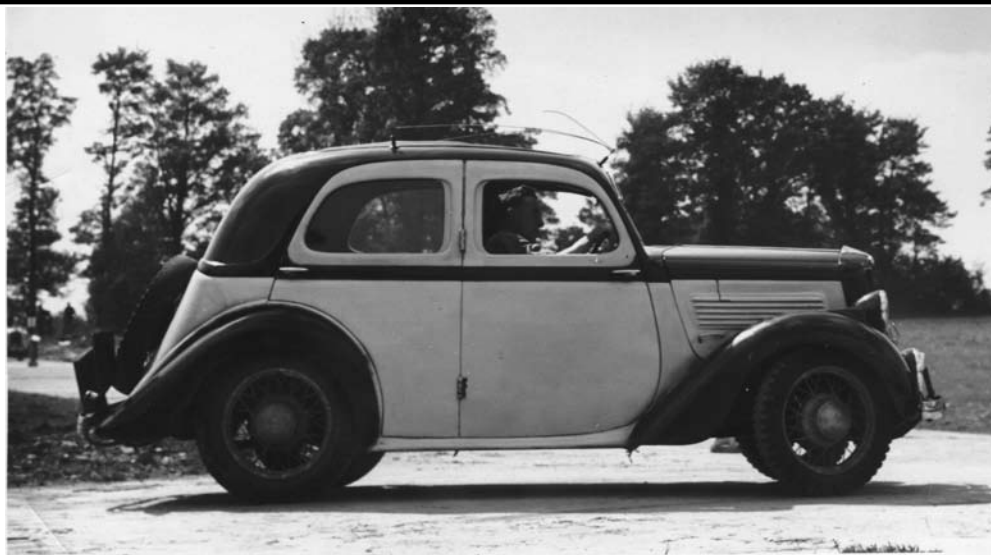
"BVX 115 on driving tests. Note radio aerial, bald spare tyre and Town and Country tyres on the front."
