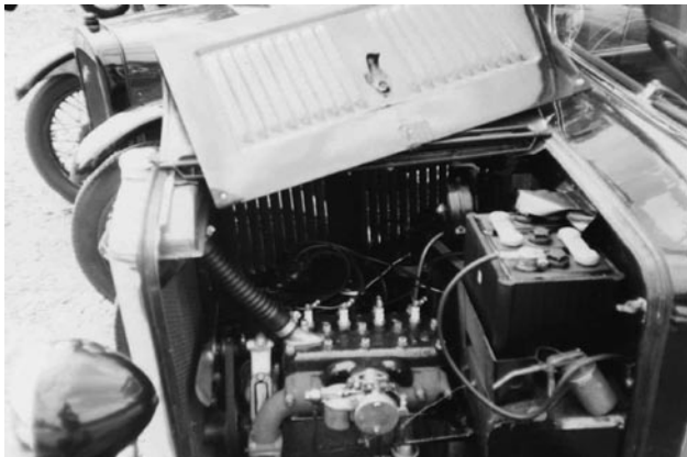
An RP Austin Seven from 1933. Polished header tank and air-intake cover are non-original. So is underbonnet battery mounting. The car belongs to Austin and Ford enthusiast, Brian Eckersley.
