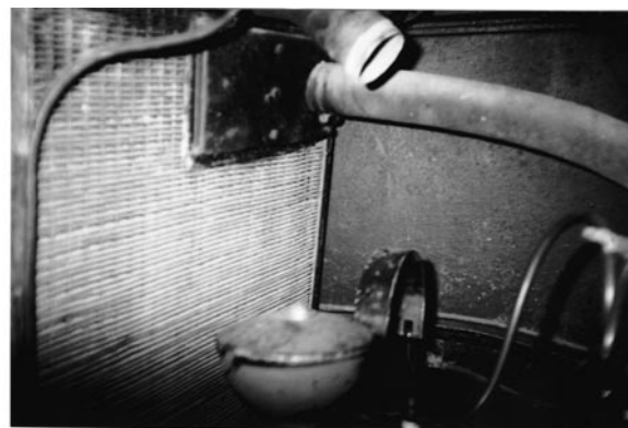
The warm air intake from the radiator core on David Bond's Ford Model Y.
