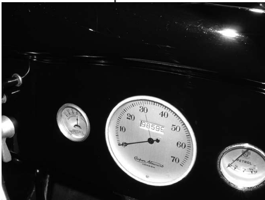
"The neat instruments of Raymond Neave's December 1935 Model Y. Note the red line denoting the 30 m.p.h. point on the speedometer. I don't think this was normal on Model Y's, but am open to correction."
