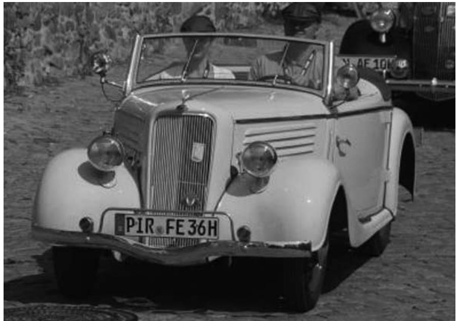
A frontal view of the Eifel Gläser roadster. Although the German caption to the original photograph states that it is a 'Gläser-cabrio', the doors do not seem to have sliding windows incorporated.
