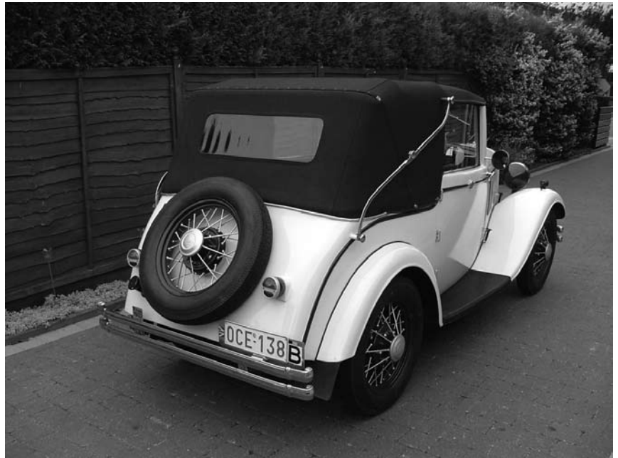
The rear view of Philip Raemdonck's Cairn showing the weather-proof Salmons Tickford hood. Note the non-standard bumper and Philip's personal number plate OCE-138."
