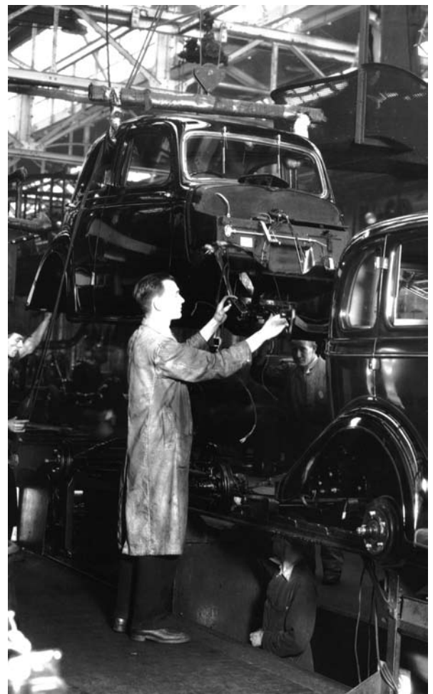
Here we see a Model 'C' body being lowered from the 'High Line' onto the production line. It is now clear that the chap guiding the body is holding the front of the chassis. The front chassis cross-member can be seen to the right of his right hand. Also, the front axle can be seen below with its transverse spring clearly free from any chassis.
