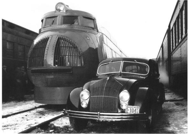
Chrysler's Art & Colour staff were responsible for the design of the Airflow body with the passengers sitting in front of the rear axle and the advanced, but infamous, 'waterfall' grille, shared by the Union Pacific locomotive.
