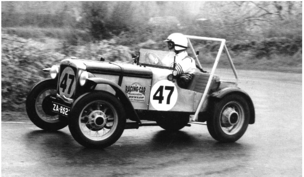
Denis in action at the Corkscrew Hillclimb in the nineties. Note the roll-cage, which quickly bolts on for competition use and cleverly incorporates mounts for the timing transponder, harnesses and rear fog lamp."
