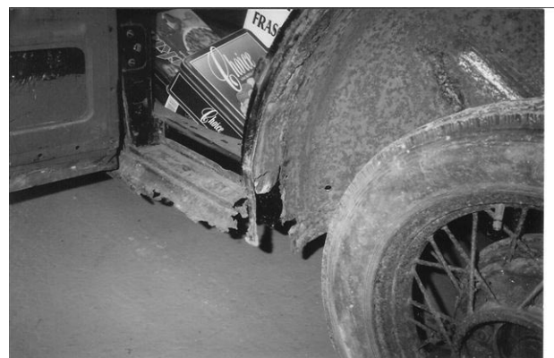
The sills had almost rotted away.
