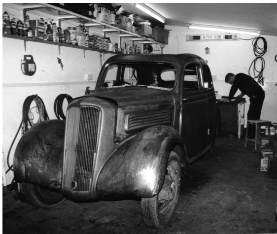
November 1992: the car is stripped bare, repaired and ready for its primer coat. The draughtsman friend tries to sketch the complicated sliding roof design
