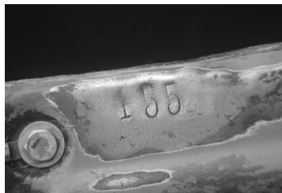
The revealed battery box assembly number 155 hand-stamped at the Ford assembly plant at Lower Hutt.
