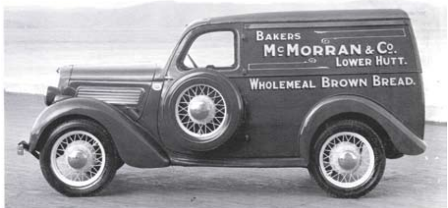
The Model "C" panel van designed and built on an imported rolling chassis by Standard Motor Bodies, Ltd., in Ebor Street, Wellington.
