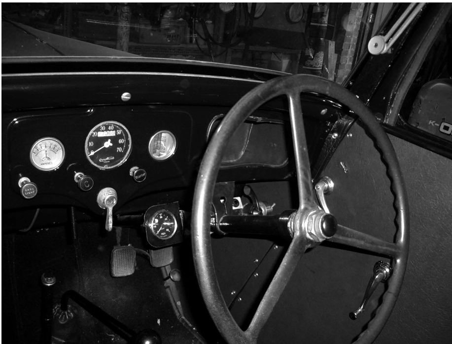
The dash board has a mix of black-faced short rad and white-faced long rad instruments and an unusual layout of choke, dash light and starter knobs. Note the added oil pressure gauge and indicator switch either side of the original steering column and wheel.
