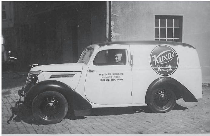
An Eijfel van (Leiferwagen), probably bodied by Papler coach-works in Cologne. Note the uncharacteristic small headlamps.
