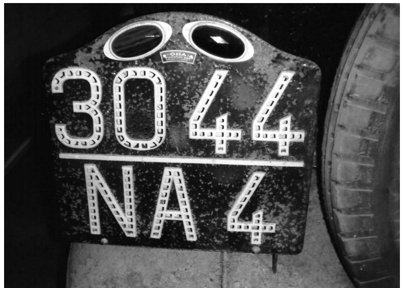
The unusual, but effective, rear number plate on Givanni's Asnières-assembled short rad. The digits and letters are picked out by reflective glass. The plate was made by ODA.
