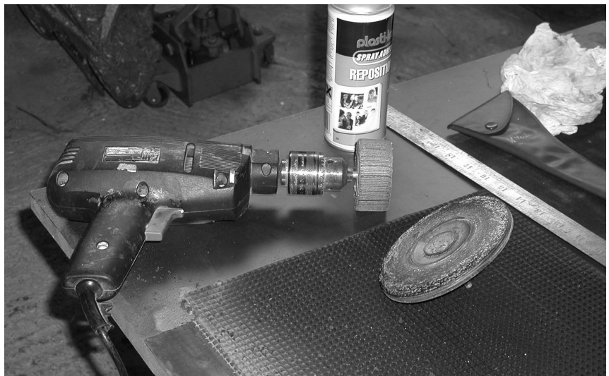
Removing the pyramids with the grinder and flap wheel.
