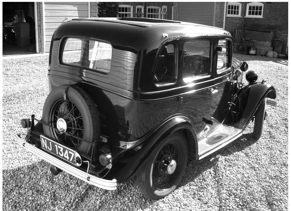
The rear view of Dave's short rad showing the Model "Y" luggage rack, the sunroof and chromed water outlets.
