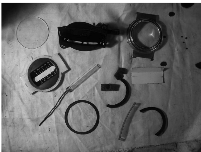
Even the gauges were stripped right down and rebuilt. Here is the hydrostatic fuel gauge in bits
