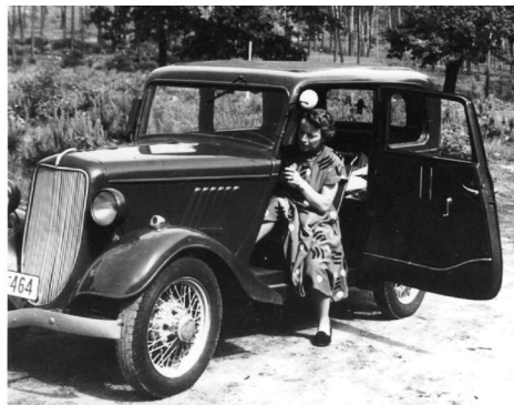
A 40-spoke wheel on a German Köln. The standard Köln wheel was the same as the Model "Y" with only 30 spokes.
