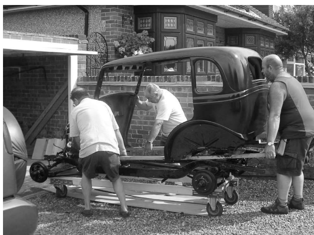
With the help of Dave and Mick, Brian guides the body onto the chassis (which has been rebuilt on top of a home-made trolley).
