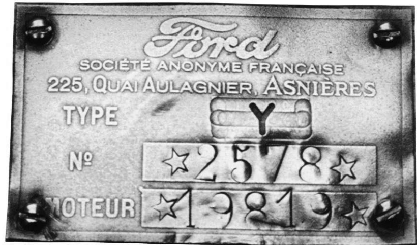
The brass plaque which was screwed to the bulkhead below the battery box on Fords assembled at Asnières, Paris.
