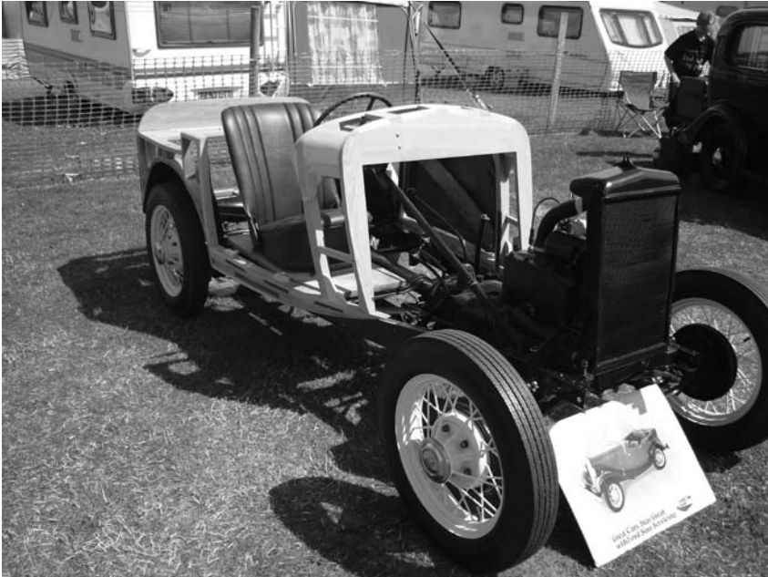
With the chassis, axles, engine and transmission already completed, Doug has expertly fabricated the woodwork of the body tub on the Abbey. Here seen at the Caerwys Show in July.
