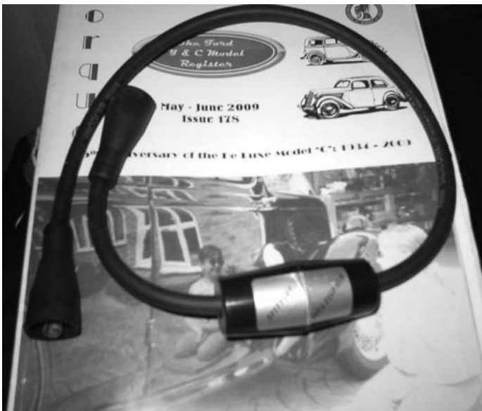
A Multispark HT lead which produces five sparks at the plug instead of the usual one, thus giving a higher efficiency and fuel saving - or so it says on the packet.
