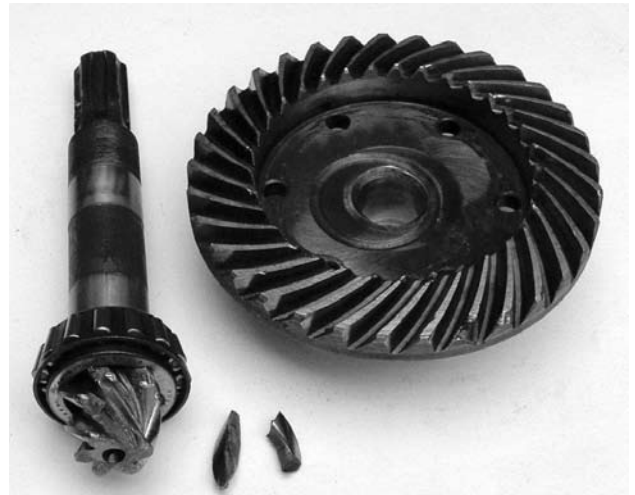
Ron was complaining of a knock in his transmission! The culprits were a couple of sheered teeth off his pinion, which also caused damage to the crown wheel
