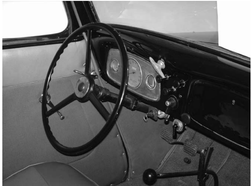
The unusual arrangement of the dip switch, which is between the brake and clutch pedals on this long rad Model “Y”, for sale in Majorca last year.
