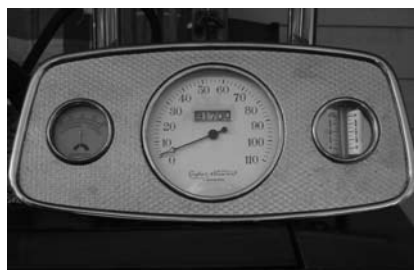
The beautifully restored engine-turned instrument panel with the Cooper Stewart speedometer readings in Kilometres per Hour.
