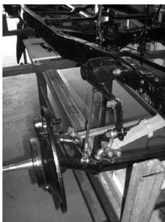
One month later, in July, the assembled nearside (LHD) front axle with original shock absorber. Note drag link appearing from the steering column and drop arm on the left hand side.
