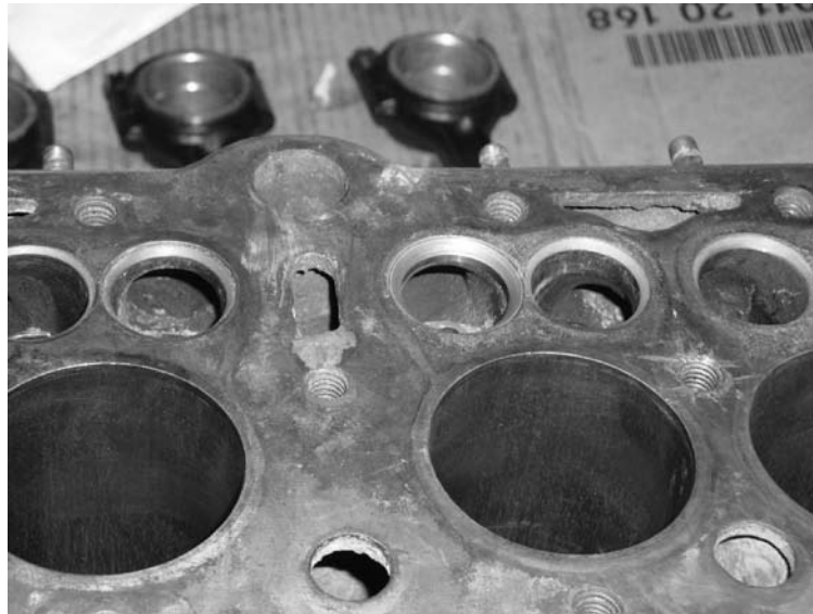
In the photograph, the newly inserted hardened exhaust seat (second) can be seen.
