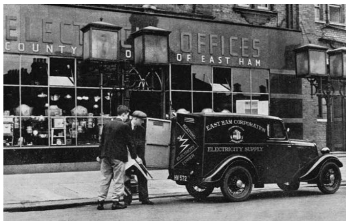
Another pre-October 1936 East Ham registered van with its spare-wheel air-brushed from the driver's door. The louvres on the rear doors are clear in this photograph.
