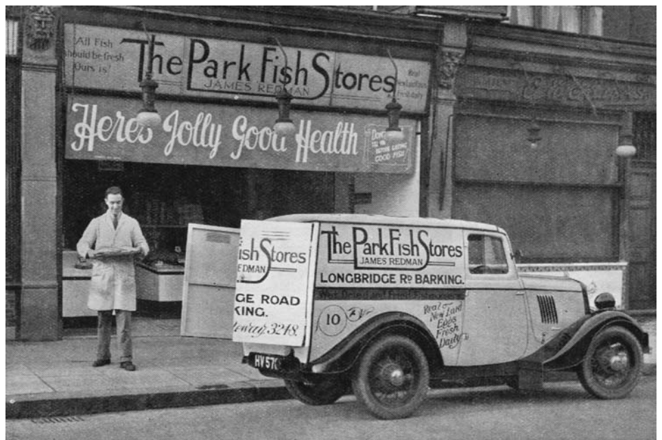
A supposed late (post-October 1936) version of the Model "Y" van with its spare wheel fitted to the near-side door. However, the HV East Ham registration dates the van at early 1936. It is suspected that, once again, 'The Ford Times' publisher air-brushed out the spare wheel on the driver's door.
