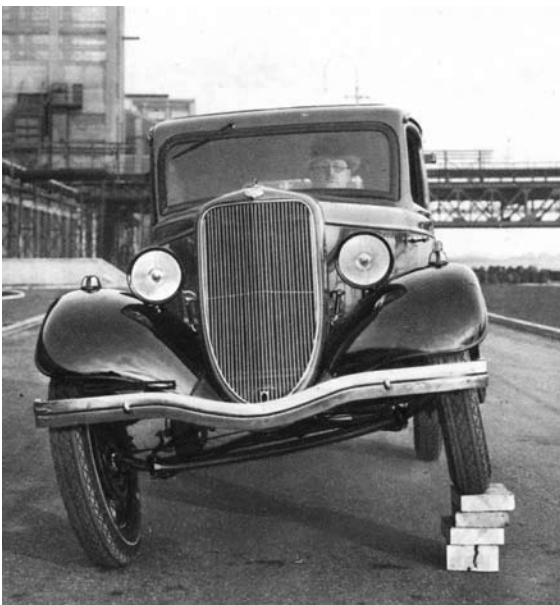
I'm sure the bespectacled trilby sitting in the passenger seat is trying to show that the body tub sits almost square on the road despite the major suspension tilt. Note the railway gantry leading off to the Dagenham jetty and building to the rear of the car."
