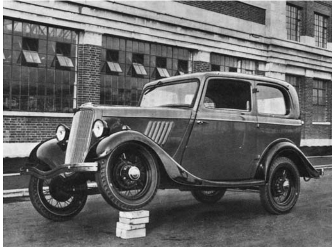
A 1934 Tudor Model "Y" demonstrates the arc of travel of the transverse suspension. Note the start of a second storey on the building behind.
