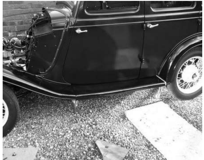
When boards are of the correct length, with packing if necessary, you can commence the fitting of the new rubber matting.
