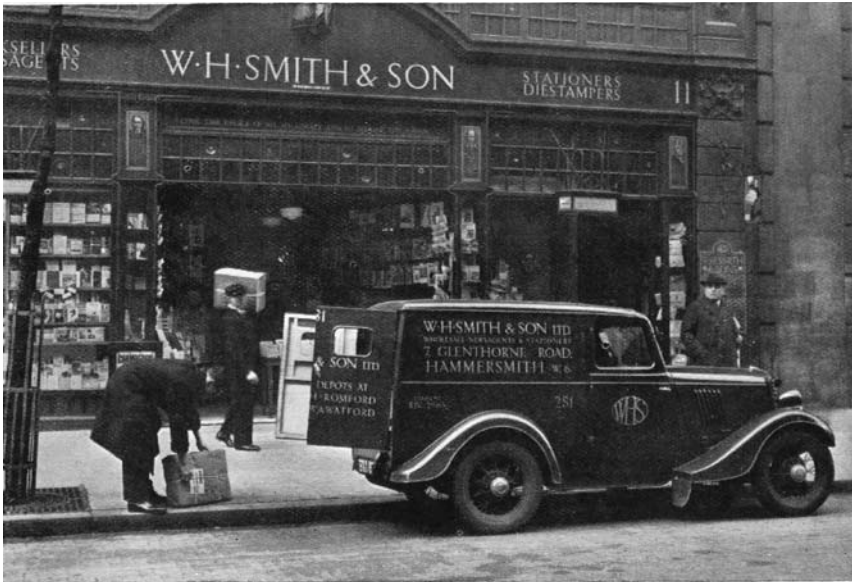
The rear doors on this van have been privately modified to include windows. Note the longer mud-flap on the front wing. Earlier vans had shorter mud-flaps
