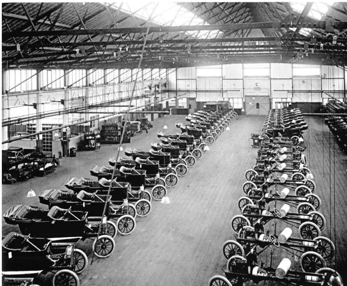
Model Ts being assembled at Trafford Park. Ford occupied what had been the tramcar factory belonging to the British Electric Car Company.
