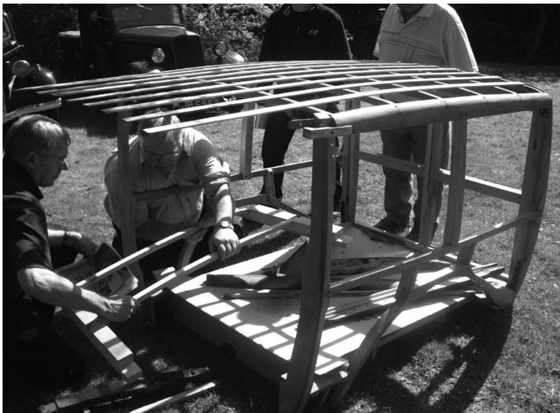
Roger Hanslip and Geoff Dee try to work out where the extra bits go on the superbly crafted 'skeletal' body built by Noel Page for Roger's van project. An envious Geoff Dee has a similar restoration project in hand!
