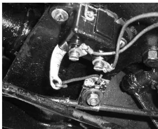
Brake light switch, YE-13480, in situ on the rear of the middle chassis cross-member (gearbox to the right). When rear foot brake is applied the clamped brake rod moves to the rear (left) pushing the lever to make contact inside the Bakelite box.
