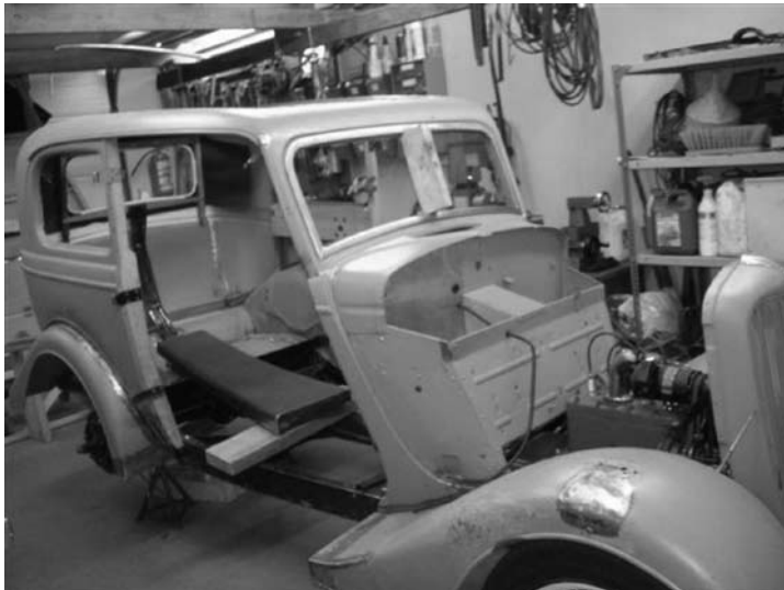
Bernt Solheim's June 1934 Tudor Model "Y" with the sawn off 1933/34 V8 Model 40 windscreen surround fitted.
